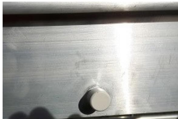
The pump has a speed control located on the irrigation tray, this is used to increase or decrease the pump speed using the + and - buttons
